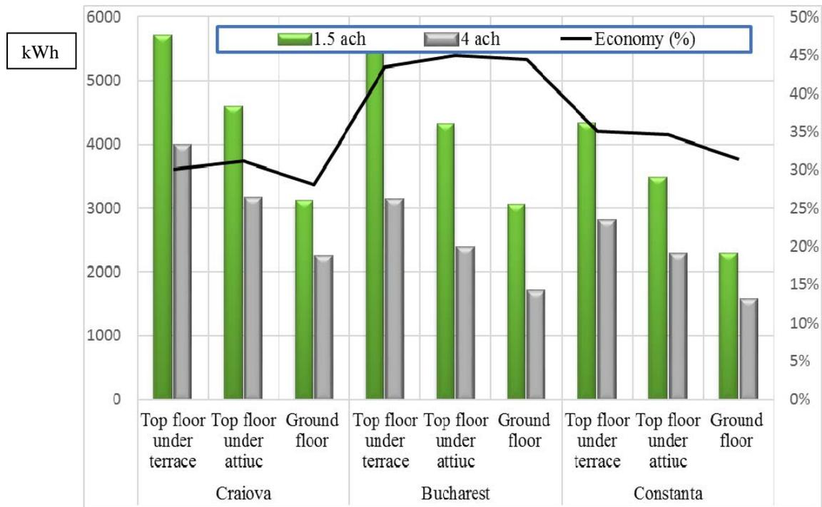
**Fig. 8** - Energy consumption for cooling and economy for different climates, different position in the building and for different night ventilation rates
