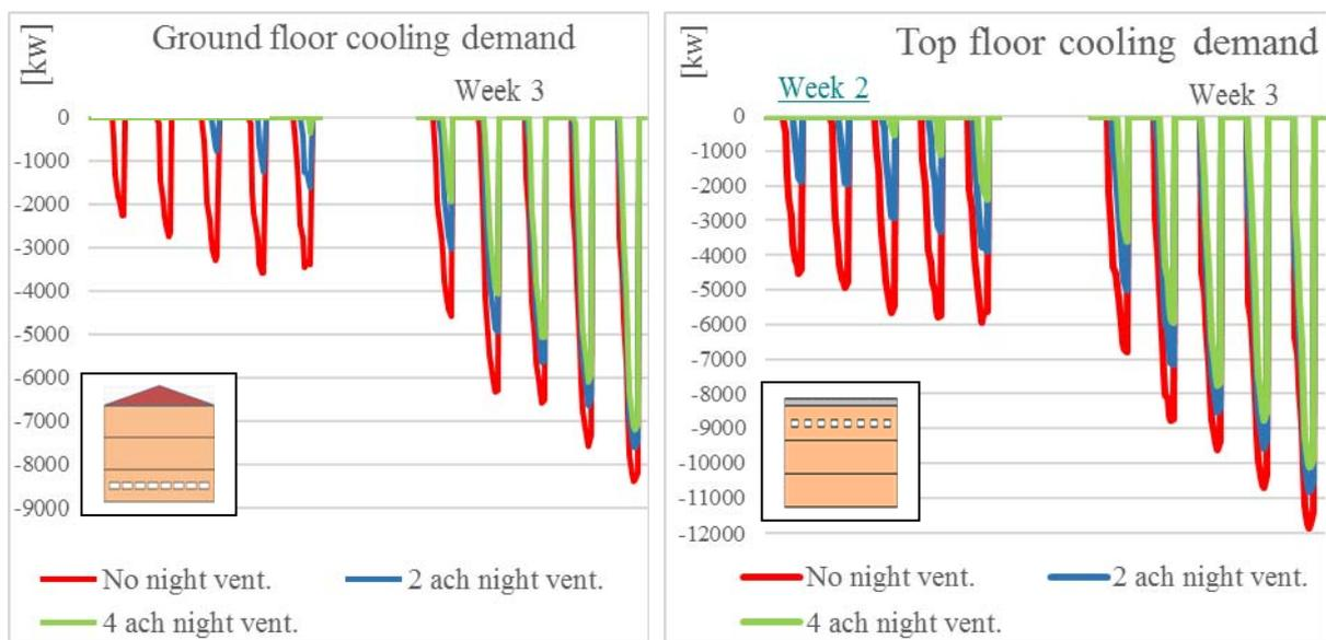
Fig.1 - Cooling demand - office top floor, Air set point=25<sup>0</sup>C
