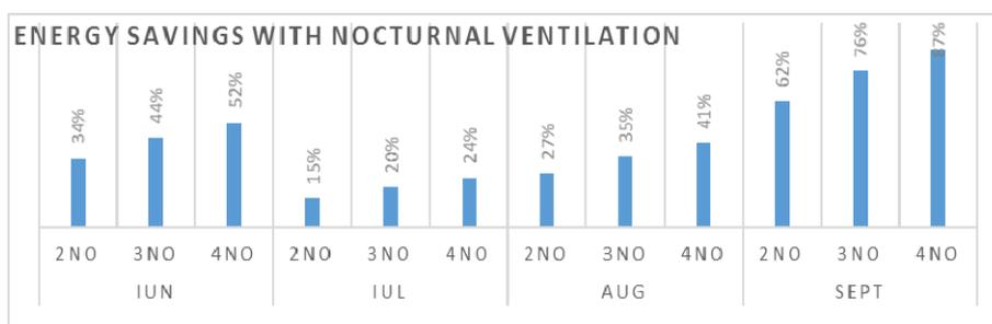
**Fig. 4** - Percentage reduction of required cooling by applying nocturnal ventilation to a top floor office for a set point of 25°C, with nocturnal ventilation in relation to the situation without nocturnal ventilation
