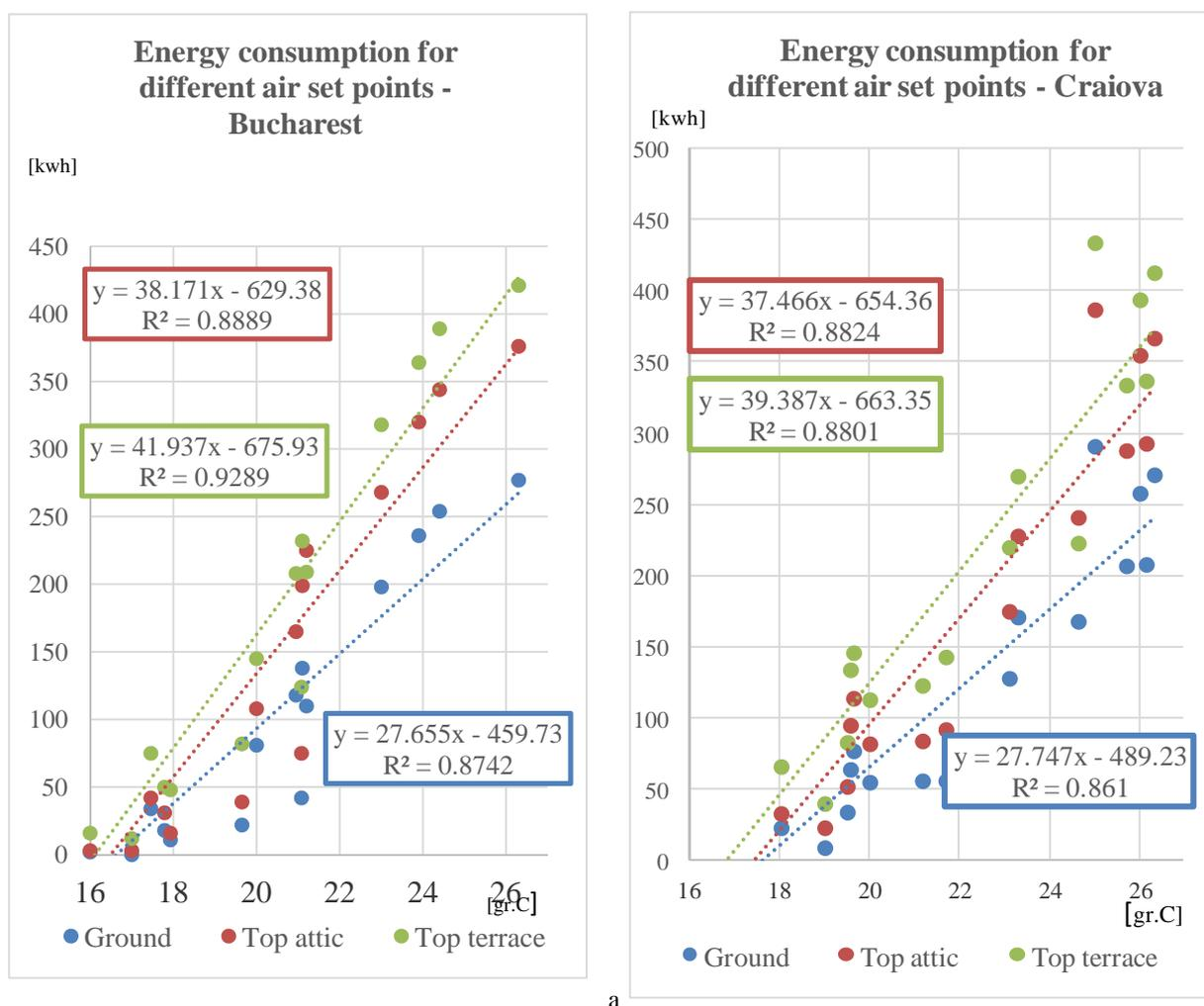
**Fig. 9** - Energy consumption for different air set points (ground – Fig. 9a and top floor – Fig. 9b)
