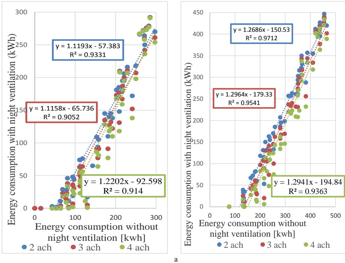
**Fig. 6 -** Cooling energy consumption relation with and without nocturnal ventilation for various types of structures (ground – Fig. 6a and top floor – Fig. 6b)
