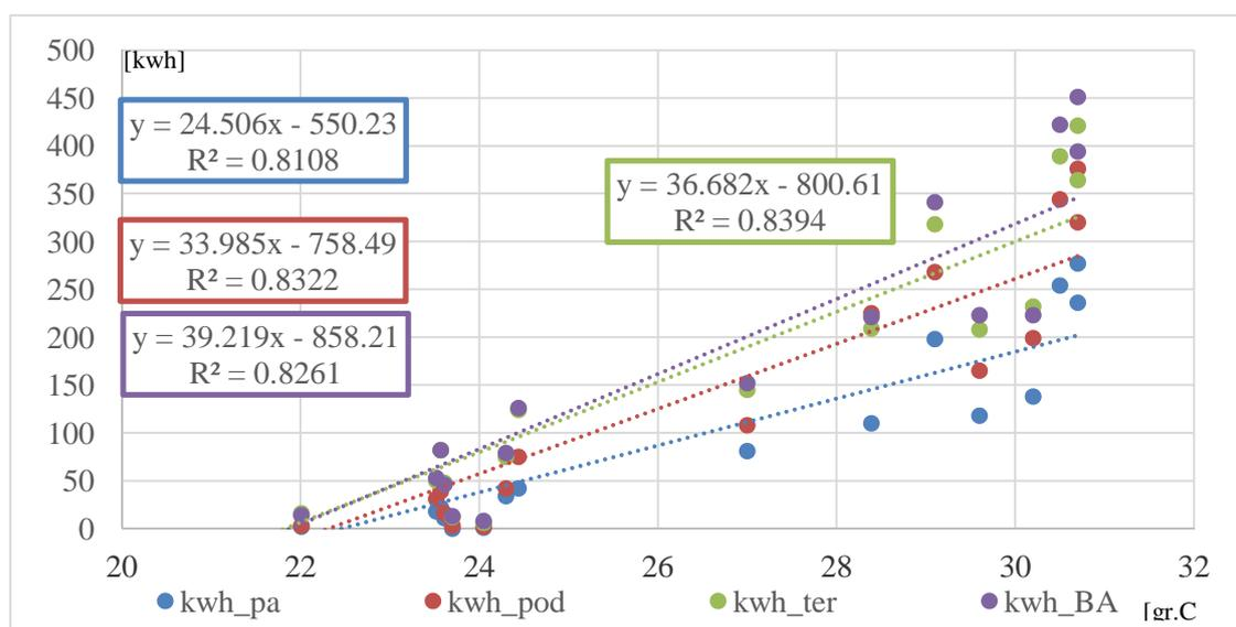
**Fig. 11** - Relationship between the indoor day air temperature and the energy consumption for Bucharest climate at nocturnal air change rate of VN=4 ach
