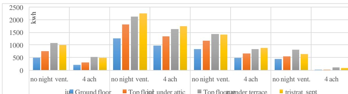
**Fig. 5**- Cooling demand in kWh based on the envelopment of the building with nocturnal ventilation (4 ach) and without nocturnal ventilation,  $t_{int}$  proposed=25°C
