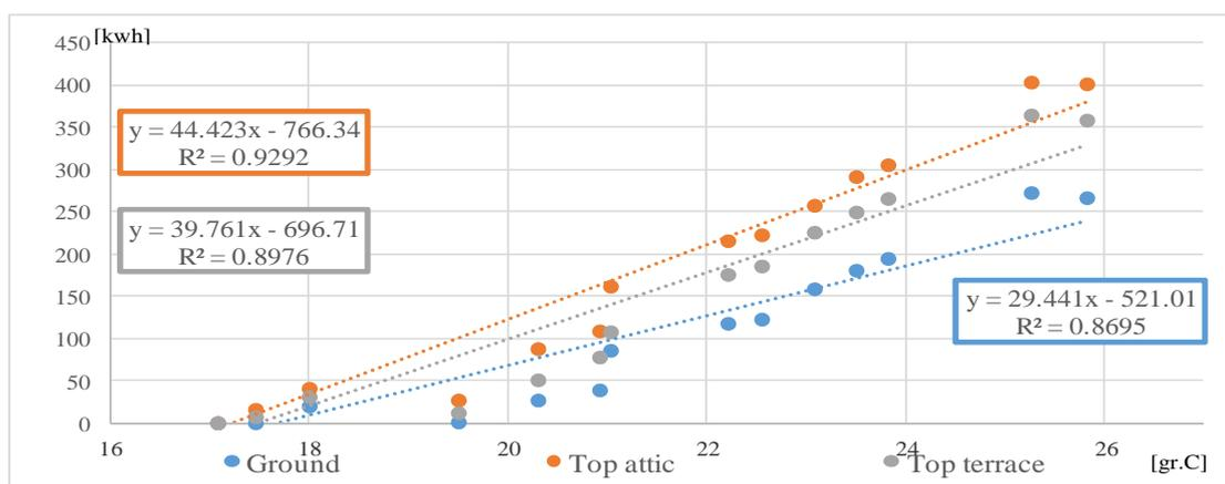
**Fig. 10** - Relationship between the indoor day air temperature and the energy consumption for Constanta climate at nocturnal air change rate of 4 ach
