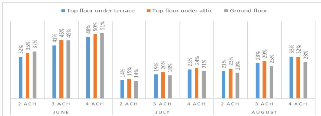
**Fig. 7- Cooling energy reduction when applying nocturnal ventilation in relation to the situation without nocturnal ventilation**
