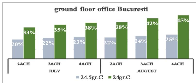
**Fig. 3** - Extra energy consumption for cooling with nocturnal ventilation for air set point temperature of 24°C and 24.5°C in relation to consumption at for air set point temperature at 25°C
